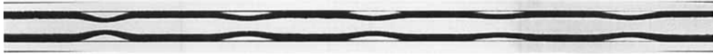
FIGURE 4. A view of the interface at 100\times magnification showing the formation of periodically spaced lobes or collars for \sigma = 173 and Ca = 0.022 . The flow is from left to right in the photograph.
